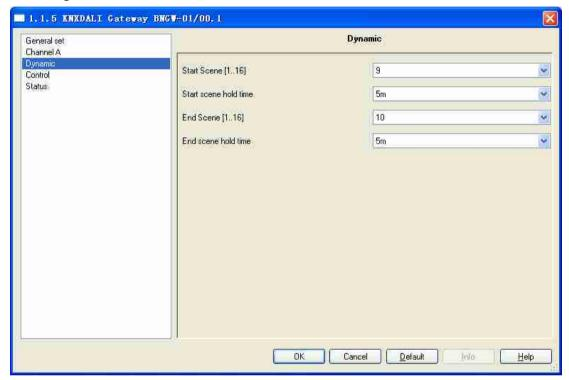
Figure 5.3 parameter settings interface "Dynamic"
