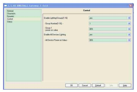
Figure 5.4 parameter setting interface "control"
